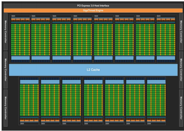
Fig. 3. Kepler GK110 full chip block diagram.
